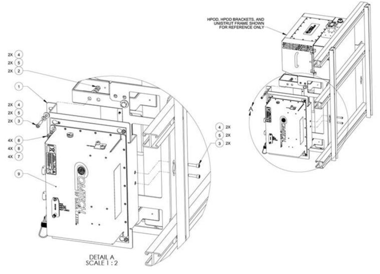
Figure A-3. Phase Combiner Box and Bracket Kit (KT-0021171)
