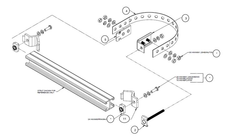
Figure A-6. HPOD 1:1 Redundancy Pole Mount Kit (PL/12319-1)
