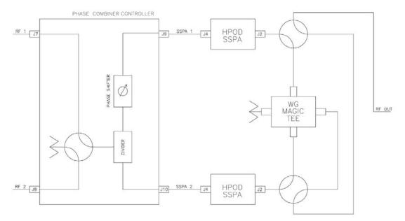
RF System Interconnect Figure 1-2. Combined System Block Diagrams
