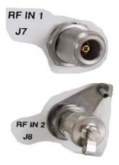
The Type 'N' **RF IN 1 | J7** and **RF IN 2 | J8** connectors serve as RF signal input interfaces to the PCCB. Note that:
