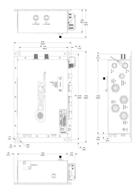
Figure 1-4. PCB-4000A Dimensional Envelope
