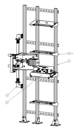
Figure A-5. Vertical Mounting Frame Kit (KT-0021179)
