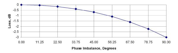
Figure 1-3. Combining Loss vs. Phase Imbalance Summary of Specifications
