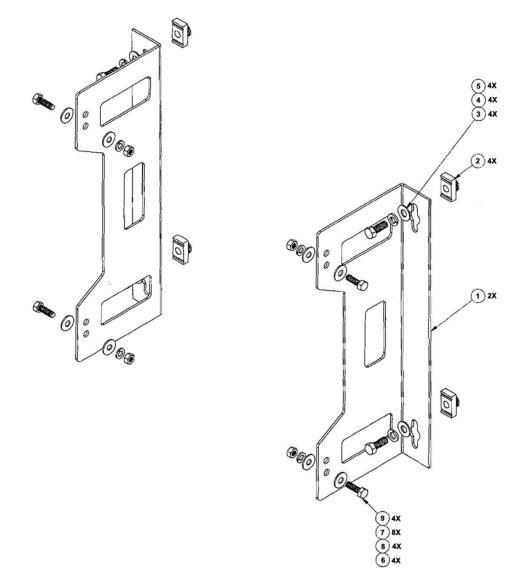
Figure A-8. Uni-Strut Mount HPOD Mounting Bracket Kit (KT/12300-1)
