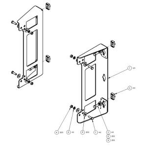
Figure A-9. Vertical Frame Uni-Strut Mount HPOD Mounting Bracket Kit (KT-0021261)
